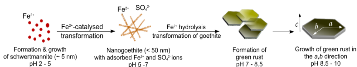
Figure 7: Schematic illustration for the formation and transformation processes involved in the formation of \text{GRSO}_4 . After (AHMED et al. , 2010).
